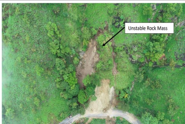
Figure 4a: Failed soil mass with rock boulders
