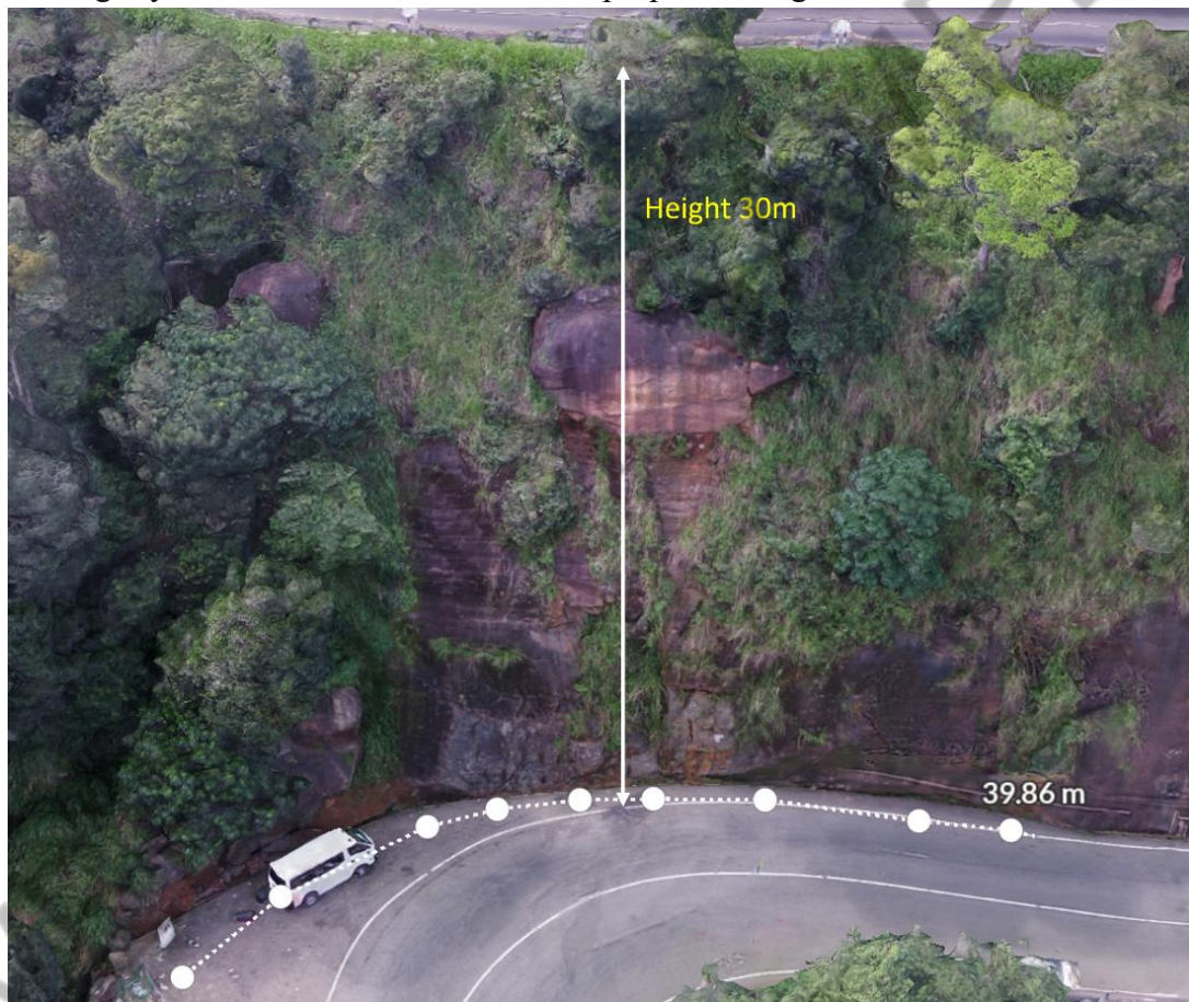
Fig 3.30: Extent of slope to be rectified (Aerial View)
