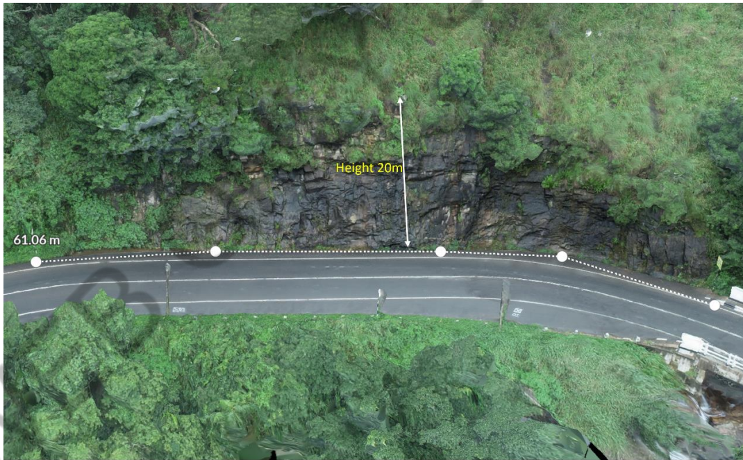
Fig 3.21: Extend of slope to be rectified at 43/8 to 43/9 (Aerial View)
