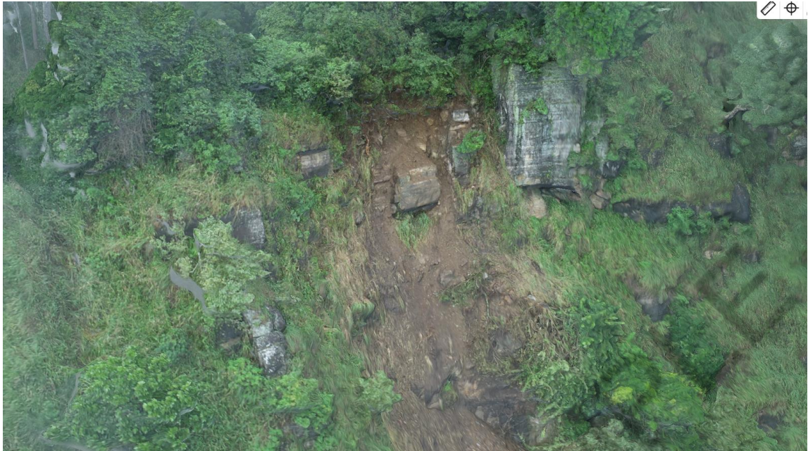
Fig 3.20: Presence of unstable boulders at 44/1 (Aerial View)
