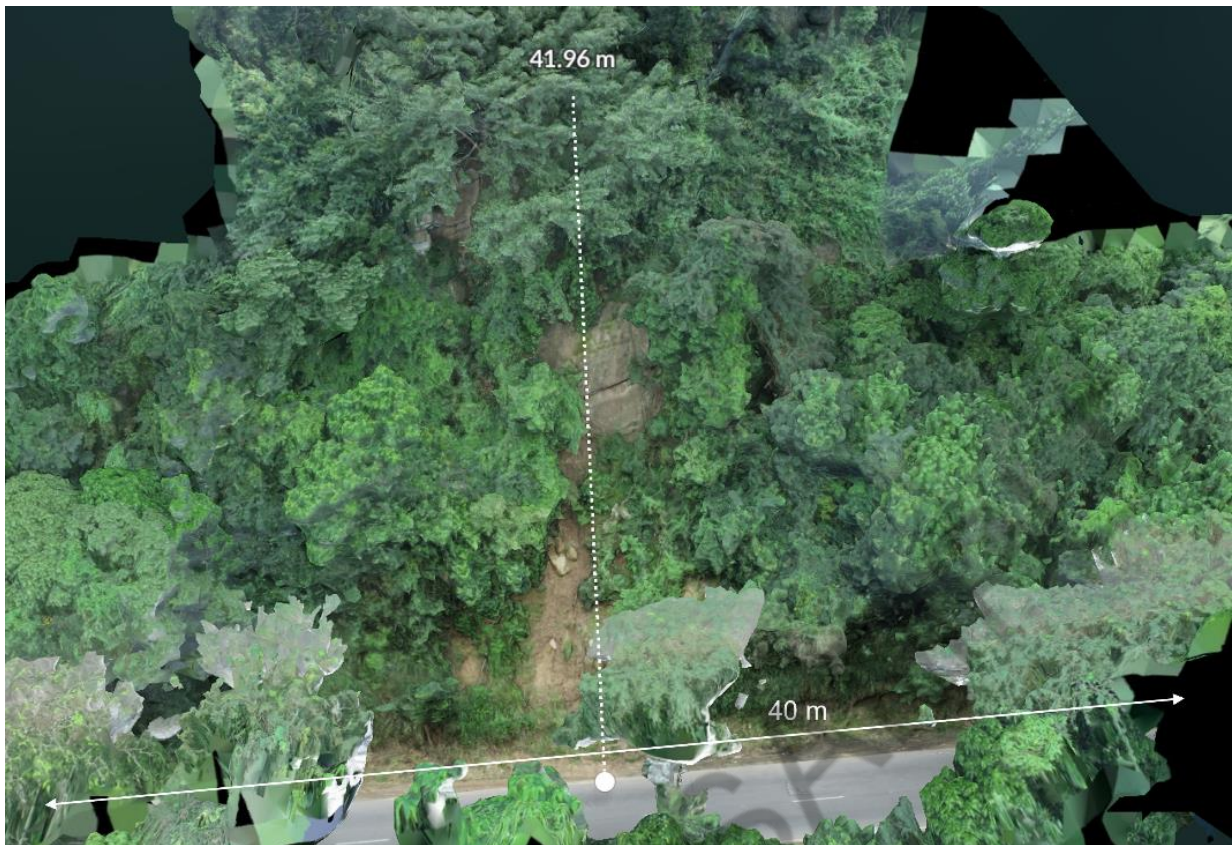
Fig 3.3: Extend of slope to be rectified between Culvert No. 17/3 to 17/4 (Aerial View)
