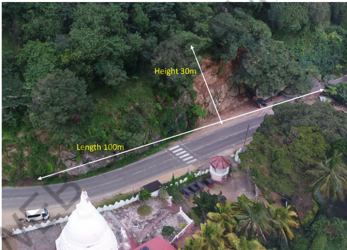
Fig 3.11: Extend of slope to be rectified
