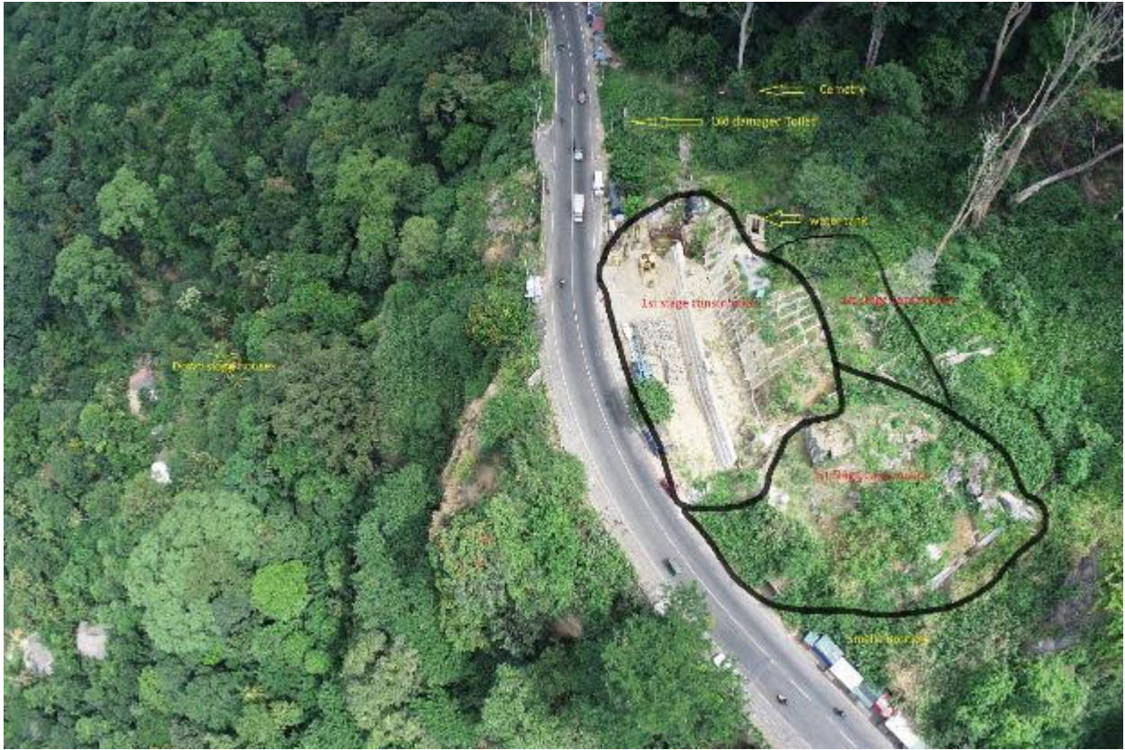
Figure 3: Drone image of the proposed landslide mitigation site, the surrounding environmental features and service infrastructure.
